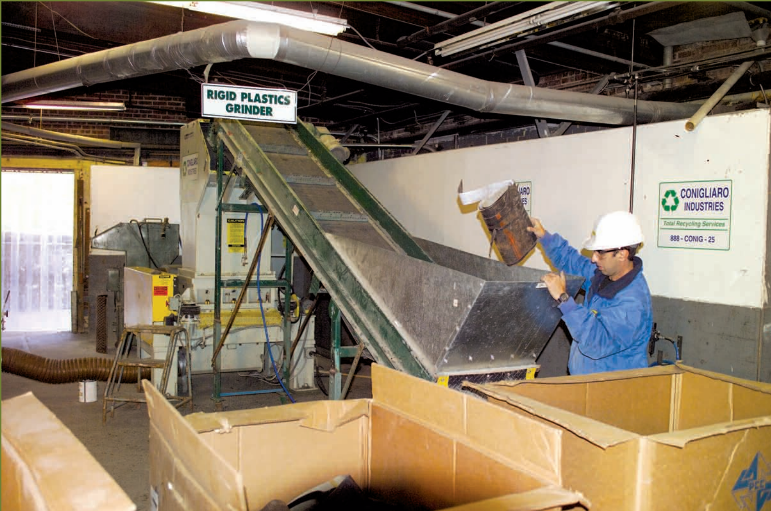
Recyclers use specialized grinding equipment to convert retired vinyl membrane to chunks or a powder. Image courtesy Vinyl Roofing Division, CFFA.
